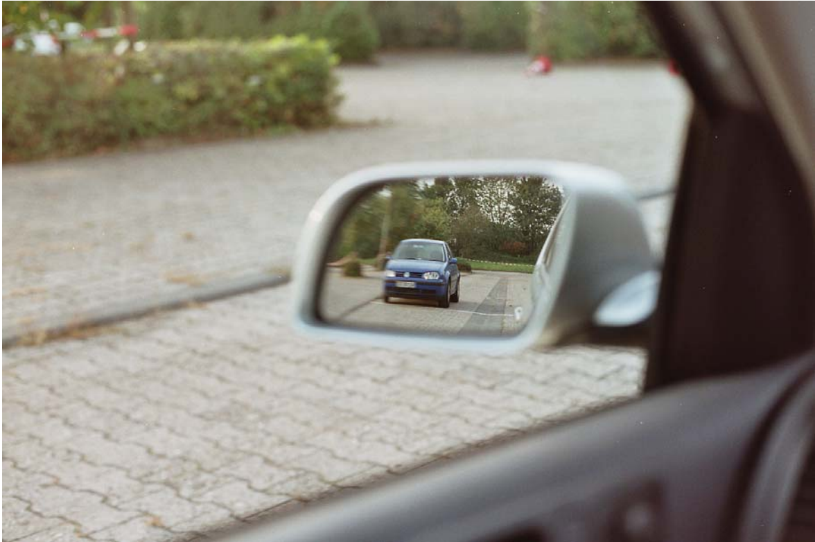
Figure 10. The view through the convex driver side mirror showing the test car B at the starting position, the beginning of the test track, and the end of the test track.
