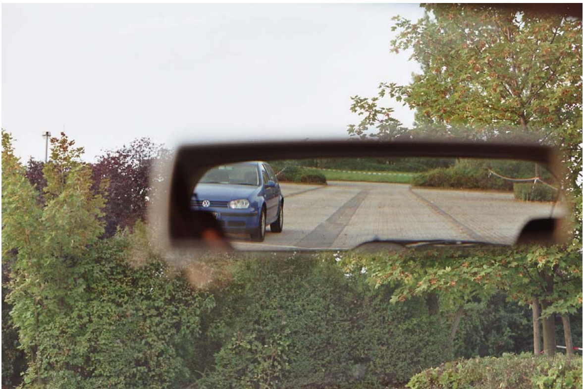
Figure 11. The view through the planar centre mirror showing the test car B at the starting position, the beginning of the test track, and the end of the test track.
