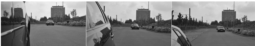
Figure 2. Example stimuli of Experiment I. Pictures show the test environment from a low (left), a conventional (middle), and a high camera position (right). In all three pictures, the first target vehicle has a distance of 30 m from the observer's vehicle and the second target vehicle a distance of 14 m from the first target vehicle.
