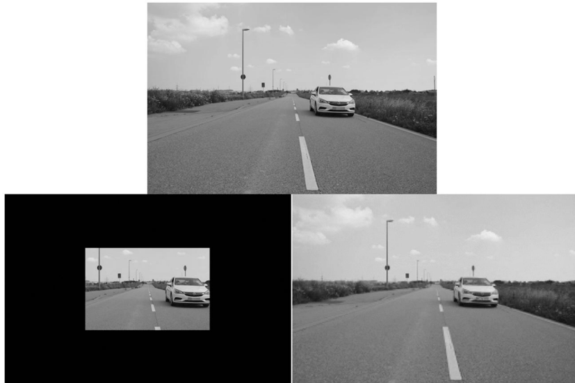
Figure 1. Example stimuli in Experiment I. All stimuli with a target distance of 10 m. The depicted environment and the image size of the vehicle are identical for all three stimuli. Top: 67° FOV, 96.4 ppi. Bottom left: 33° FOV, 96.4 ppi. Bottom right: 67° FOV, 19.3 ppi. The cropped images made the vehicle look nearer.
