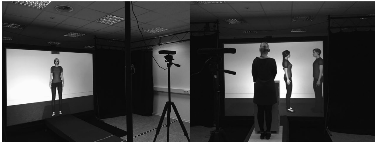
Fig. 1. Left: Apparatus used in Experiment 1 with rear projection screen displaying the avatar, platforms, and Microsoft Kinect motion tracker. Right: Setup of Experiment 2 with rear-projection screen showing the avatars, platforms, and desk in front of the subject.
