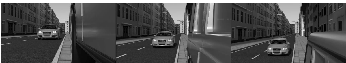
Fig. 3. Final frames of the videos used in the experiments. The vehicle is at a simulated distance of 10 m and a simulated TTP of 1 s. The camera is placed 0.5 m (left), 1.2 m (middle) or 1.9 m (right) above the ground. All videos were 1.5 s long.
